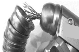
FIGURE 1. Frayed cable. DO NOT USE
