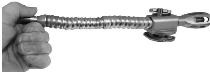
FIGURE 4. Tightened arm should hold its own weight from the distal end.
