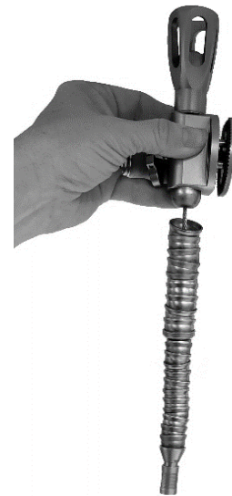
FIGURE 3. Completely loosen the arm with the main handle and dangle. Check for cable fray between every link.
